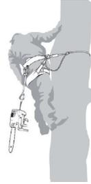
When moving the saw from any attachment point to another, operators should ensure it is secured in the new position before releasing it from the previous attachment point.
