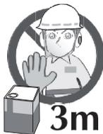
4. Always use caution when handling fuel. Wipe up all spills and then move the chain saw at least 3 m from the fueling point before starting the engine.
