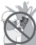
(3) Make certain that the area in which you are cutting is free from obstructions. Do not let the nose of the guide bar contact a log, branch, or any other obstruction which could be hit while you are operating the saw.
